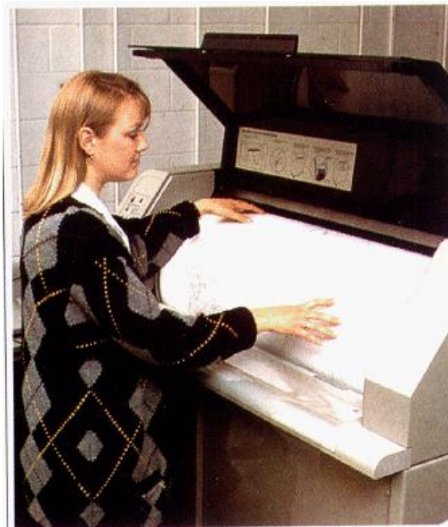
Figure 8. An electronic scanning device will convert some types of map information to digital form.
